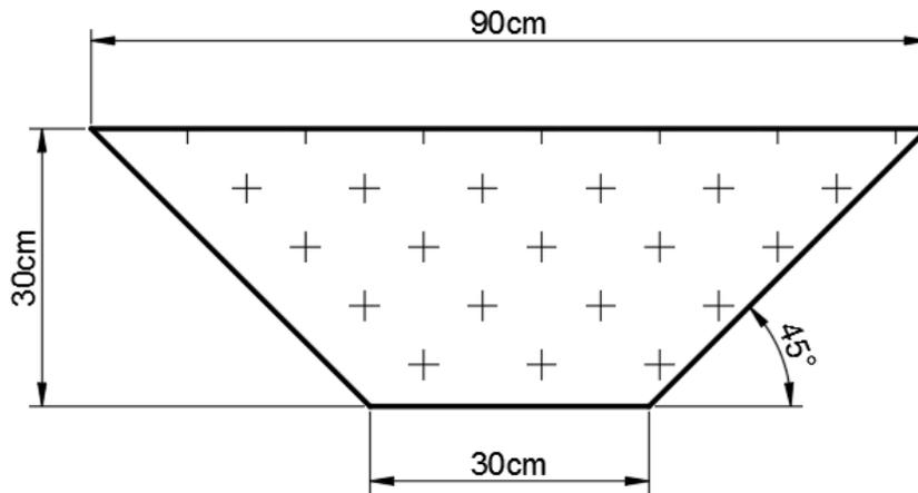
Figure 7. Surface water channel section
