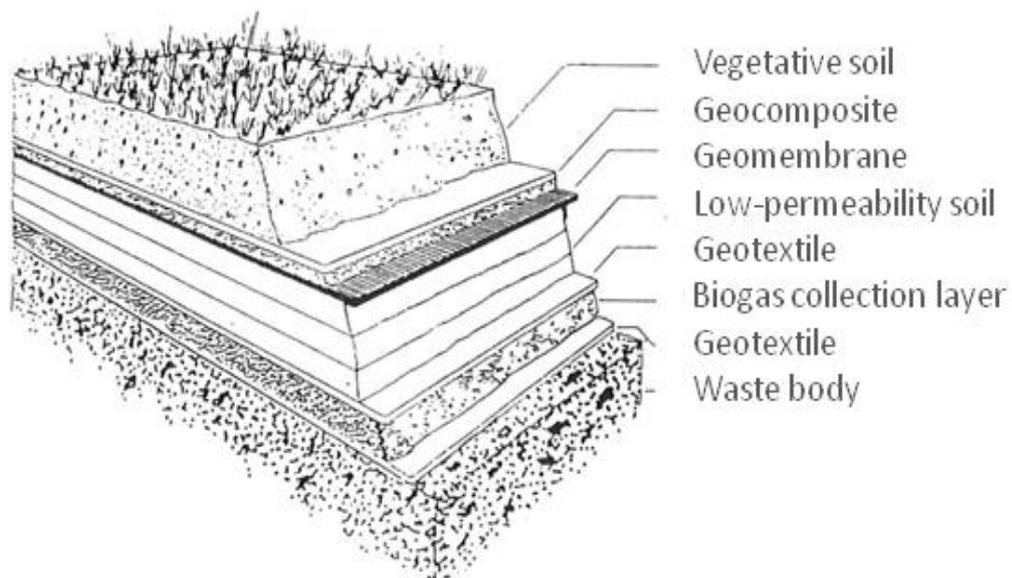
Figure 4.18. Example of landfill capping system. Source: Leachate management from Urban Solid Waste Landfill, Collivignarelli C., C.I.P.A.
