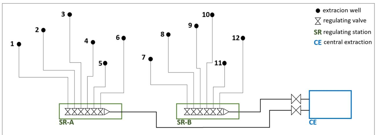
Figure 4.5. Typical framework of a landfill gas transport system. Source: adapted from Magnano E., ed. 2010, Landfill Biogas, EPC.
