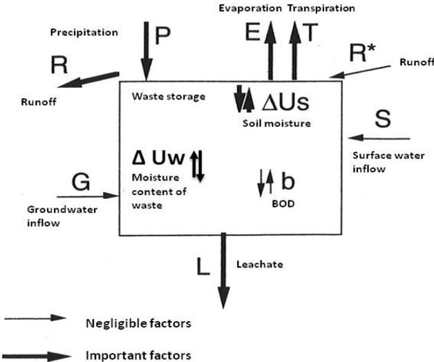
Figure 4.17. Simplified diagram of MSW landfills water balance. Source: Collivignarelli C., ed.1996, Leachate management from Urban Solid Waste Landfill, C.I.P.A
