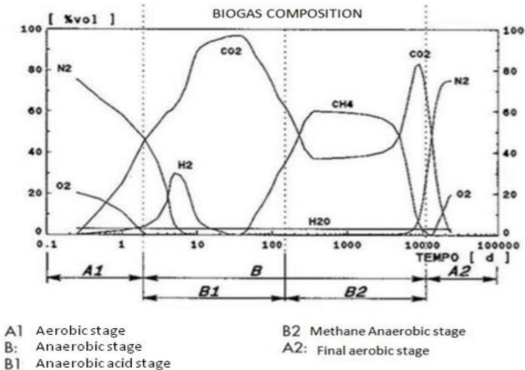
Figure 4.2. Composition process of biogas in a Landfill. Source: Damiani L., Gandolla M., 1992, Biogas management in controlled landfills, Istituto per l'Ambiente.
