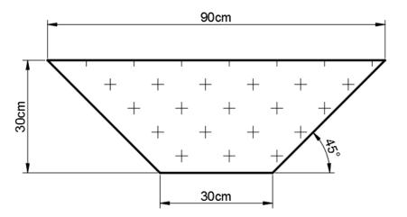
Figure 7. Surface water channel section
