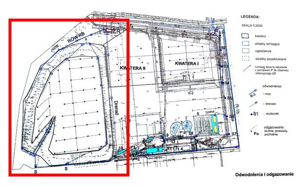
Fig. 4. Scheme of the open dumps with drainage markings and a drainage and degassing system [1].
