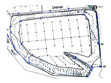
Figure 10. Scheme of degassing points of the open dumps (view from the west side) [1].
