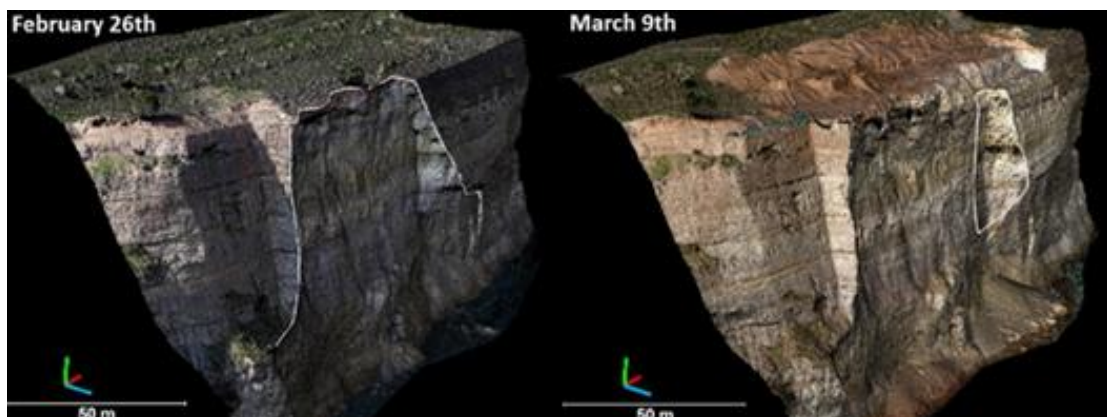
Figure 3.23. Pix4d presentation of the point cloud showing the slope failure in the Corinth Canal that took place on February 26 and March 9.
