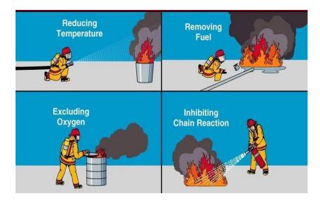
Figure 4.3. Fire extinguishing techniques.
