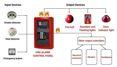
Figure 4.7. Fire alarm control panel.
