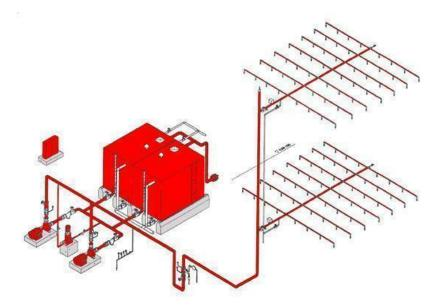
Figure 4.8. Sprinkler system.
