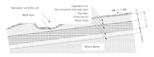
Figure 4. The capping system of Basin 1 – Stratigraphy- Source: Donini A., Pelonghini L., ed. 1998,2004, Geological-geotechnical reports carried out on the occasion of the projects for the construction of the leachate lagoon and the reservoir lake.
