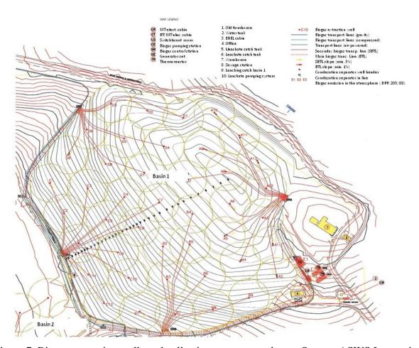
Figure 7. Biogas extraction wells and collection systems – scheme. Source: ASWS International, May 2003, Final Environmental Recovery Project - Biogas Capture and Combustion Facility with Energy Recovery Basin1.
