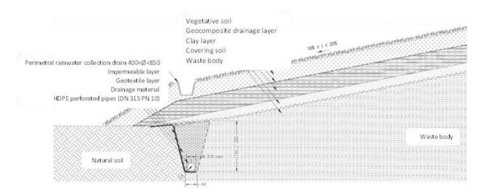
Figure 6. Drainage trench surrounding Basin 1- detail. Source: Donini A., Pelonghini L., ed. 1998,2004, Geological-geotechnical reports carried out on the occasion of the projects for the construction of the leachate lagoon and the reservoir lake.
