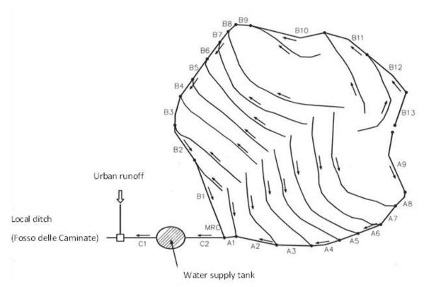
Figure 5. Collection network of meteoric water - Basin 1. Source: Donini A., Pelonghini L., ed. 1998,2004, Geological-geotechnical reports carried out on the occasion of the projects for the construction of the leachate lagoon and the reservoir lake
