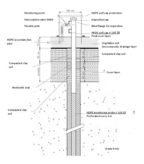
Figure 8. Biogas extraction tube drilled into Basin 1- detail. Source: ASWS International, May 2003, Final Environmental Recovery Project - Biogas Capture and Combustion Facility with Energy Recovery Basin
