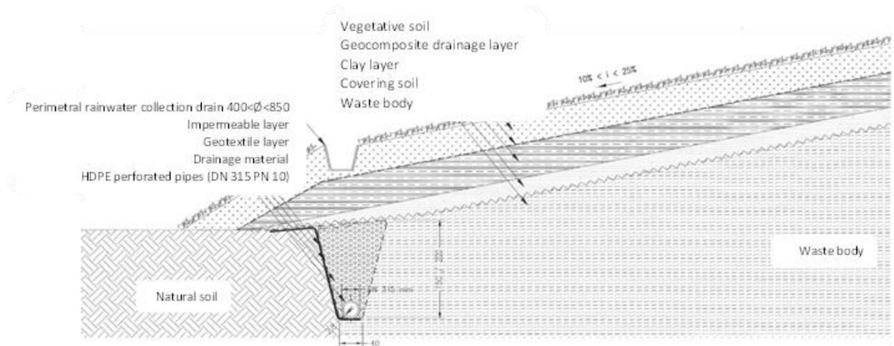
Figure 6. Drainage trench surrounding Basin 1- detail. Source: Donini A., Pelonghini L., ed. 1998,2004, Geological-geotechnical reports carried out on the occasion of the projects for the construction of the leachate lagoon and the reservoir lake.
