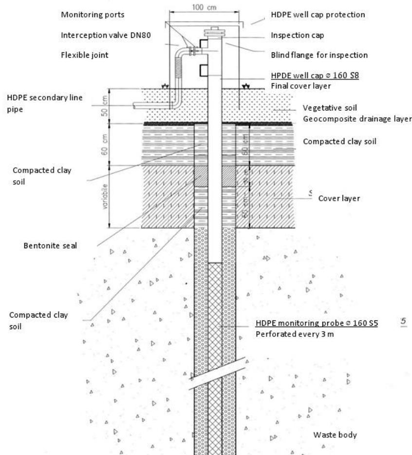
Figure 8. Biogas extraction tube drilled into Basin 1- detail. Source: ASWS International, May 2003, Final Environmental Recovery Project - Biogas Capture and Combustion Facility with Energy Recovery Basin
