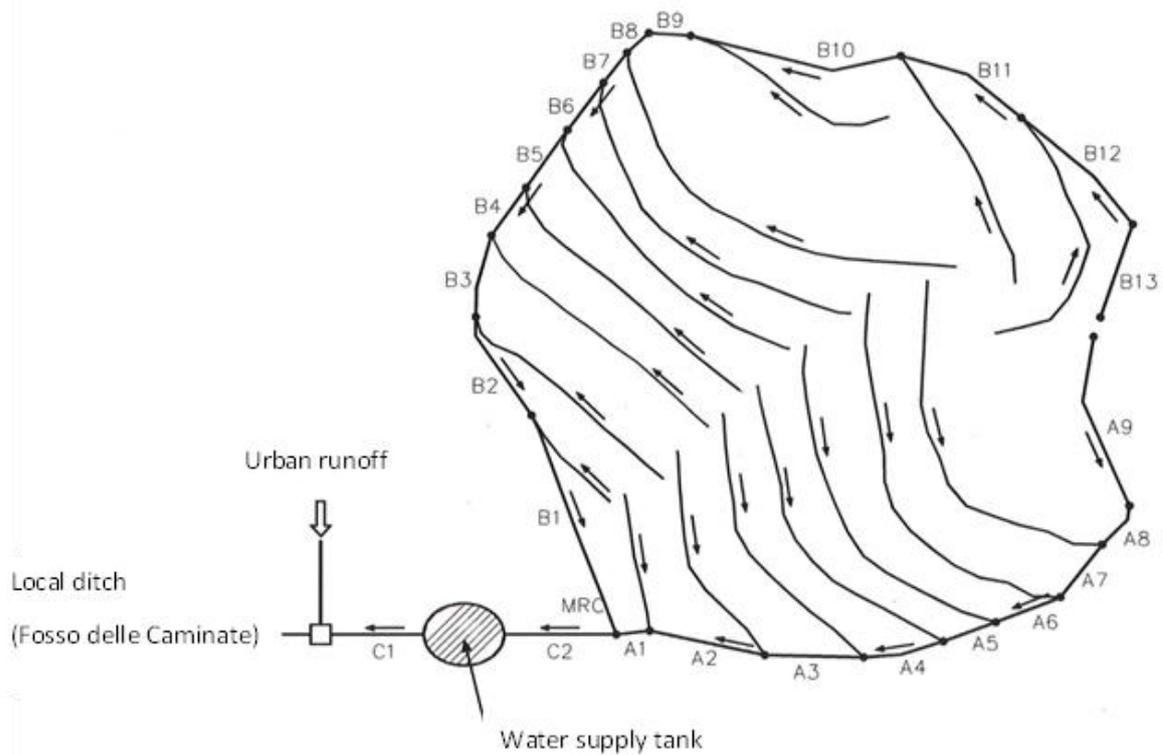
Figure 5. Collection network of meteoric water - Basin 1. Source: Donini A., Pelonghini L., ed. 1998,2004, Geological-geotechnical reports carried out on the occasion of the projects for the construction of the leachate lagoon and the reservoir lake
