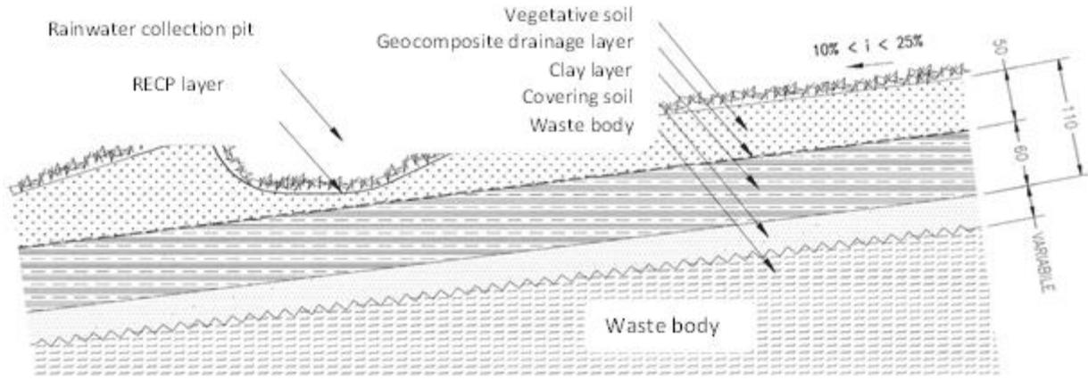
Figure 4. The capping system of Basin 1 – Stratigraphy- Source: Donini A., Pelonghini L., ed. 1998,2004, Geological-geotechnical reports carried out on the occasion of the projects for the construction of the leachate lagoon and the reservoir lake.
