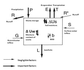
Figure 4.17. Simplified diagram of MSW landfills water balance. Source: Collivignarelli C., ed.1996, Leachate management from Urban Solid Waste Landfill, C.I.P.A
