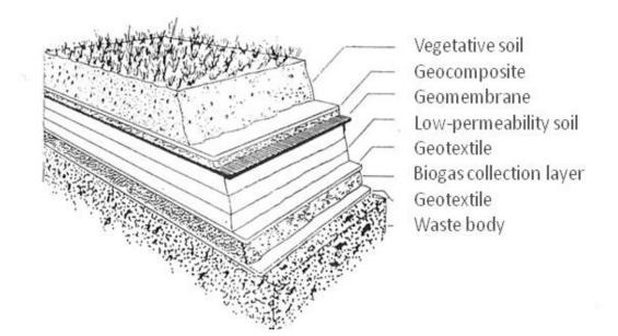
Figure 4.18. Example of landfill capping system. Source: Leachate management from Urban Solid Waste Landfill, Collivignarelli C., C.I.P.A.
