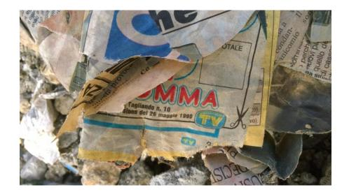
Figure 4.1. Paper Waste after 30 years of deposition. Source: ASET Spa, October 2016
