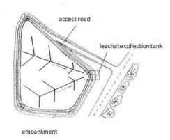
Figure 4.16.Typical scheme for leachate drainage in a controlled. Source: The controlled landfills, Gervasoni S., ed 2000, HOEPLI
