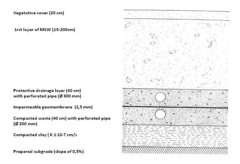
Figure 4.13. A traditional MSWL design cross section. Source: Gervasoni S., ed 2000, The controlled landfills, HOEPLI
