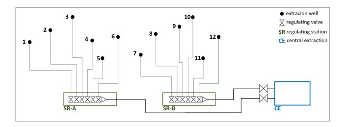
Figure 4.5. Typical framework of a landfill gas transport system. Source: adapted from Magnano E., ed. 2010, Landfill Biogas, EPC.
