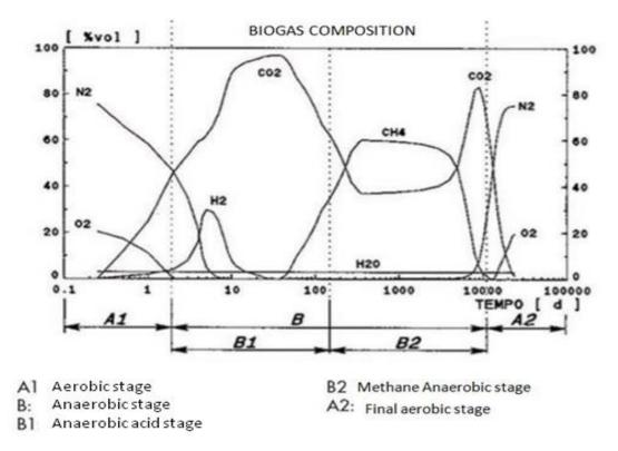
Figure 4.2. Composition process of biogas in a Landfill. Source: Damiani L., Gandolla M., 1992, Biogas management in controlled landfills, Istituto per l'Ambiente.
