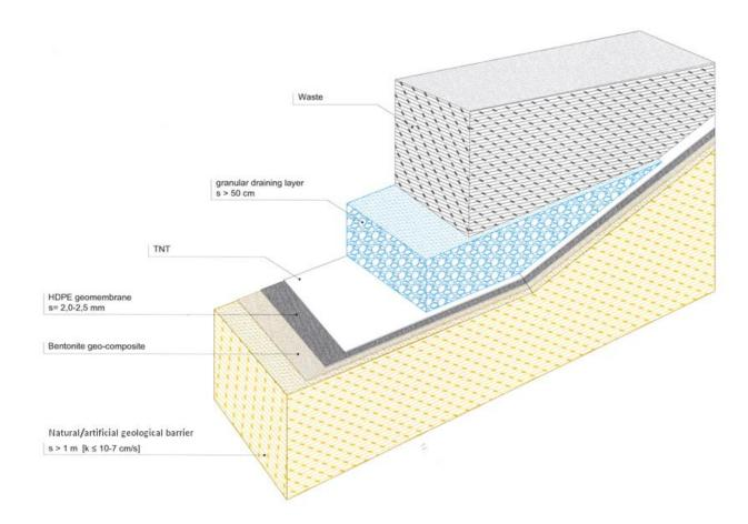
Figure 4.14. Example of different geomembranes associated with geotextile. Source: ASET Spa, 2022.
